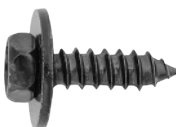
21839 (Toyota: 90159-A0001; 90159-50316) Zinc M5.2-2.0 x 21mm (#12 x 13/16") Phillips Hex Head Sems® Washer Outer Diameter: 14mm (9/16") Hex: 10mm Front Bumper, Bumper Stay & Radiator Grille Toyota & Lexus 2000 - On UNIT PACKAGE: 25
