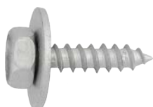
25238 Zinc Dacromet Phillips Hex Head Sems® Tapping Screw M5-2.12 x 22mm Hex: 10mm Washer Diameter: 18mm Drive: #3 Phillips General Purpose
