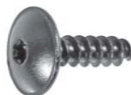
21541 (13144822) Black Zinc M5.5 x 20mm (12 x 25/32") Torx® Truss Head T-20 Drive Head Outer Diameter: 15mm (19/32") Use with 21539 & 21540 GM 2011 - On; Saab 2003 - On UNIT PACKAGE: 25
